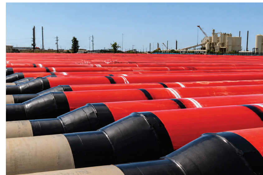
Figure 1. Onsite molded pipe ready for deepwater installation.
