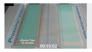
Side by side infusion of Proxxima™ R3100 and a standard infusion epoxy. After 53 seconds, the Proxxima<sup>™</sup> panel has fully infused. The epoxy panel infusion is complete after 17 min 43 sec.
