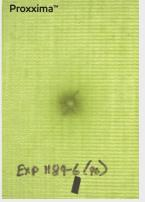
Falling weight impact ASTM D7136-07
